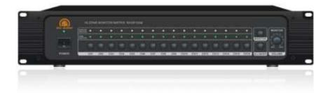
The <u>RH AUDIO</u> 16-zone speaker selector switch RH2813AM has 4 channel inputs (A1,A2,A3,A4) of amplified signal for BGM, with 4 channel inputs (B1,B2,B3,B4) of amplified signal for paging, and 16 individual relay switches, allows the user to distribute an amplified speaker signal up to 16 listening zones.
