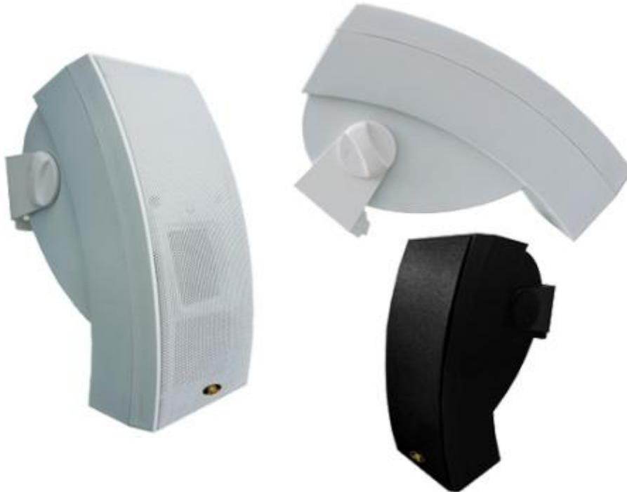
The [RH-AUDIO](#) Fashionable Voice Evacuation System Speaker RH-MS85 comes with unique and outstanding appearance design, this pa loudspeaker employs unparalleled 2 way speaker system with typically 8 Ohms low to middle frequency 4 inch driver and two 2.5 inch tweeters. Like the other constant-voltage speakers the RH-MS85 is also built in a step-down transformer to match the divers' impedance.
